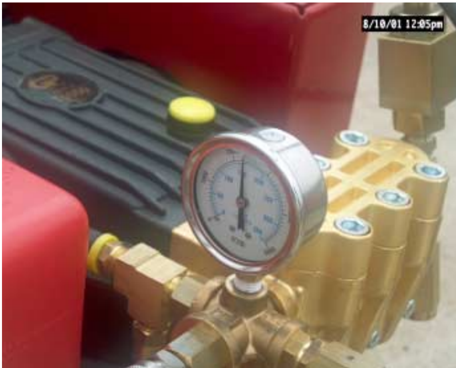
Figure 15. Gage to monitor outlet pressure from washer pump on the KY 551 bridge over Green River Lake in Adair Co.
